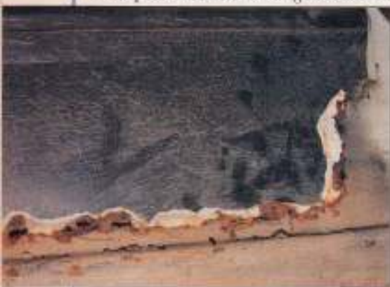
Lower edges of doors (and tailgate/bootlid) may be virtually non-existent. Usually the most cost-effective solution is to find a secondhand panel in better condition if the rest of the car is sound.
