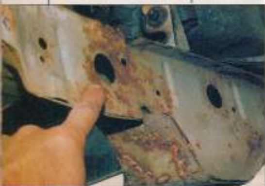
Front crossmember and surrounding structure are usually hidden by engine. However, closely inspect the vitally important steelwork here. If corrosion is widespread look for another car.
